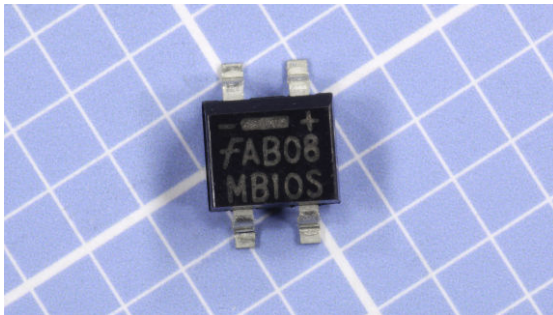
Figure 26-14. This surface-mount component contains four diodes forming a full-wave bridge rectifier circuit, and can pass 0.5A continuous current. It measures approximately 0.2" square.
