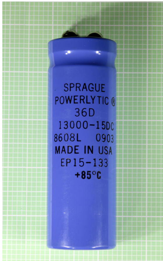
Figure 12-11. This 13,000 \mu F electrolytic capacitor is larger than would be required in most everyday applications.
