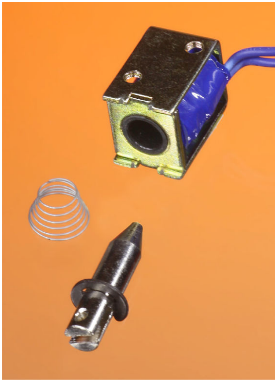
Figure 21-2. A larger solenoid rated for 24VDC.
