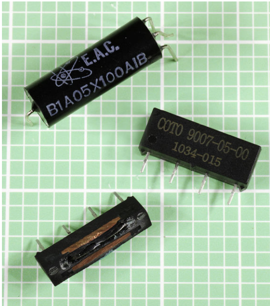
Figure 9-8. Three reed relays, one of which has had its packaging partially removed by a belt sander to reveal its copper coil and internal contacts.
