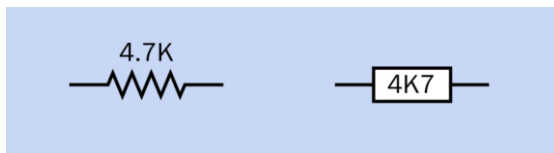
Figure 10-1. Resistor symbols. The left one is more common in the United States, while the right one is widely used in Europe. The 4.7K value was chosen arbitrarily.
