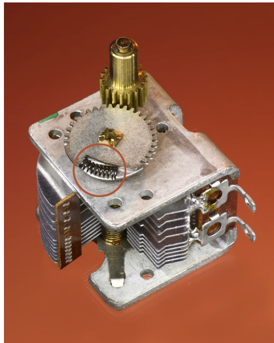
Figure 13-3. A “traditional style” variable capacitor of the type designed to tune radio frequencies. The spring, circled, enables anti-backlash gearing.
