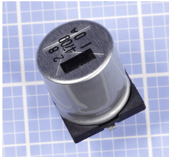
Figure 12-8. Most surface-mount capacitors are as tiny as other surface-mount components, but this 4,700\mu\text{F} electrolytic (at 10V) has a base approximately 0.6" square. A solder tab is visible at the center of the nearest edge.
