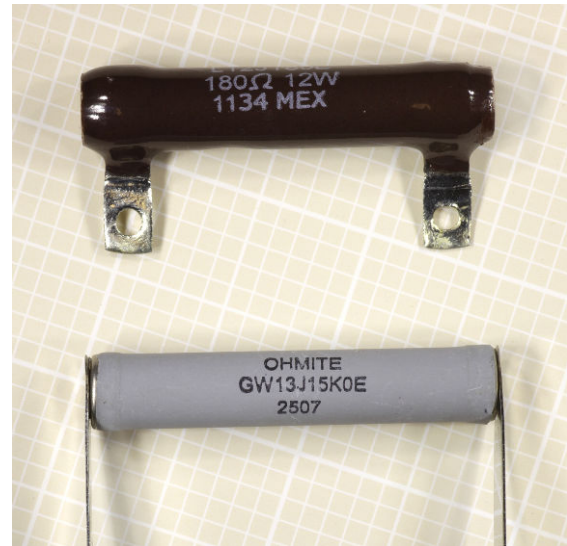
Figure 10-11. Two wire-wound resistors of greatly differing resistance but similar power dissipation capability.
