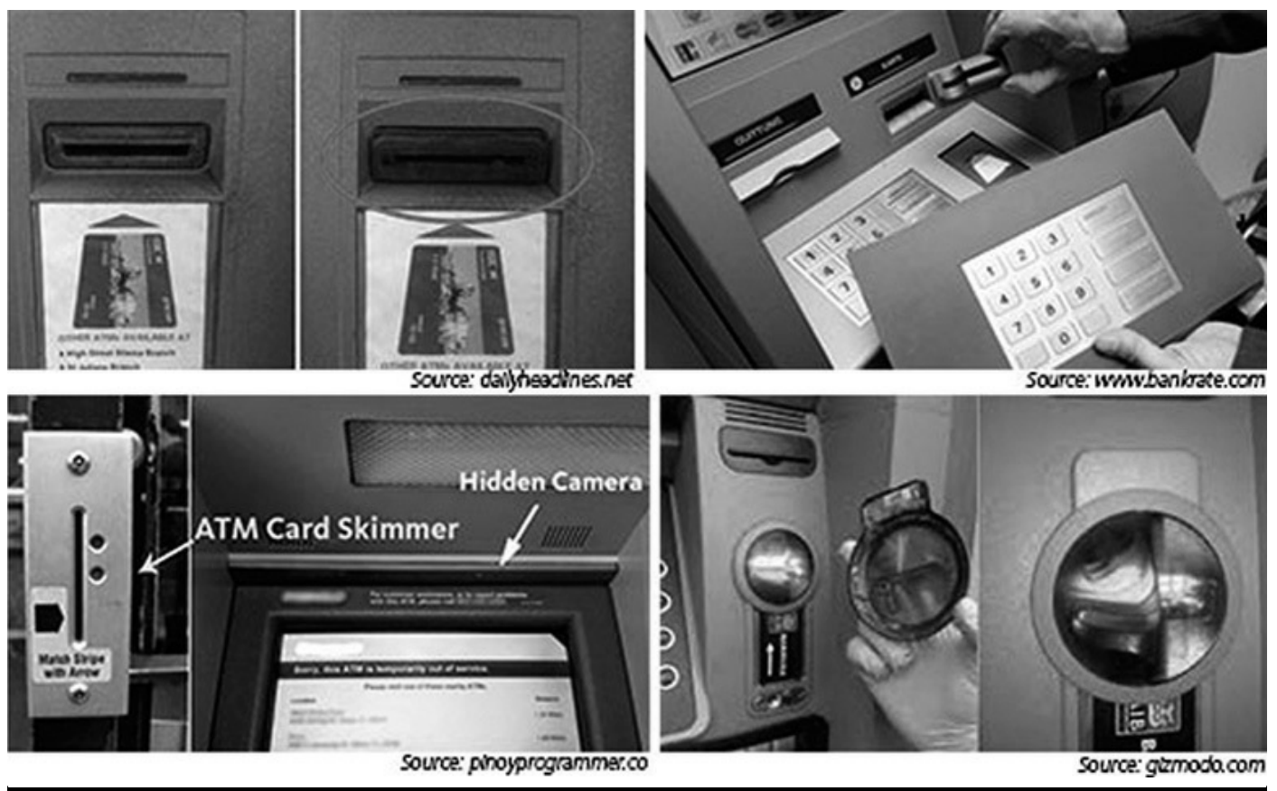
Figure 20-6 Skimmers attached to ATMs
