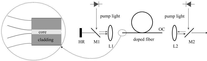
Fig. 5.40 Schematic of the experimental setup of a fiber laser
