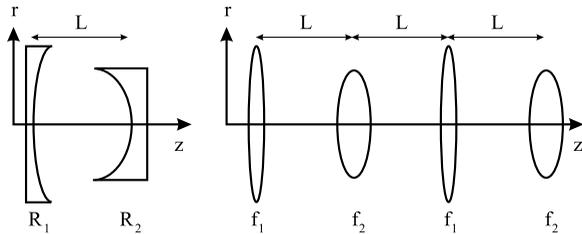
**Fig. 3.4** Fundamental element of the periodic infinite-lenses representation of a resonator
