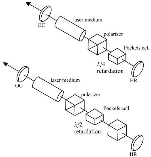
**Fig. 4.11** Setup of a cavity-dumped ruby laser [3]
