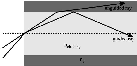
**Fig. 5.34** Path of a light ray coupled into the cladding of a fiber
