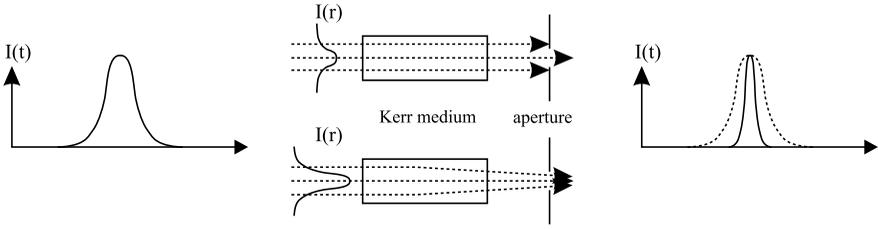
**Fig. 4.19** Kerr-lens mode-locking
