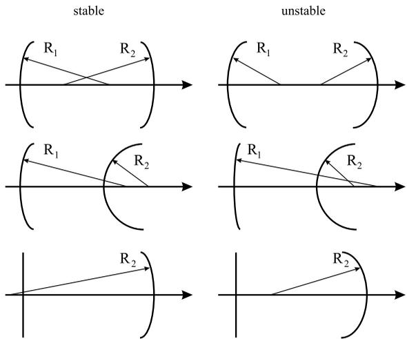
**Fig. 3.6** Stability diagram of a two-mirror resonator [2]
