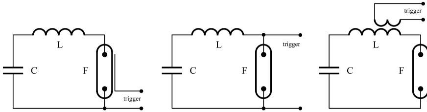
Fig. 5.7 Schematic of simple externally-triggered flashlamp circuits
