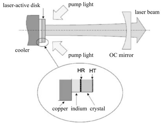
**Fig. 5.49** Mechanical design of the disk heat sink with water-jet cooling [47]
