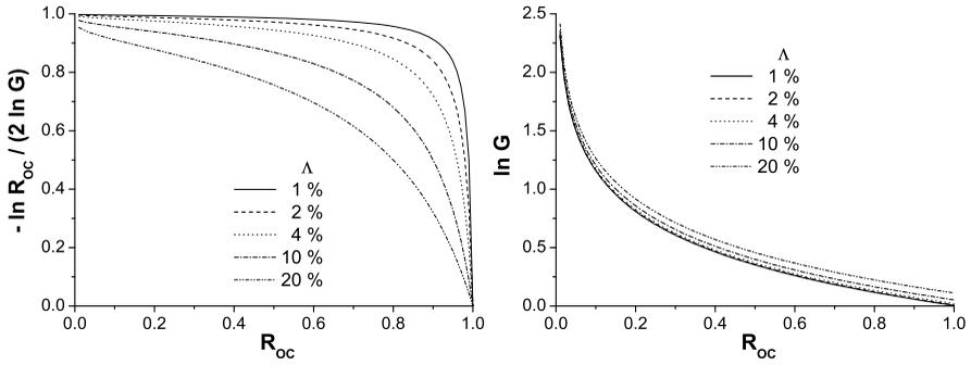
**Fig. 2.11**  $\frac{-\ln R_{OC}}{2 \ln G}$  and  $\ln G$  as a function of the output coupler reflectivity  $R_{OC}$  and the internal cavity losses  $\Lambda$
