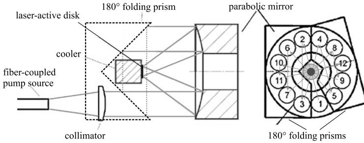
**Fig. 5.50** Schematic of the pump system of a disk laser, using a parabolic mirror and retro-reflecting prisms to achieve a total 24-pass ( $m = 12$ ) propagation of the pump radiation [47]
