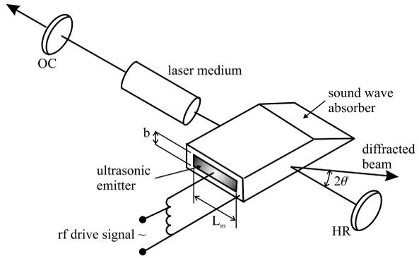
**Fig. 4.8** The two operation regimes of an acousto-optic modulator: The Raman-Nath regime and the Bragg regime [3]
