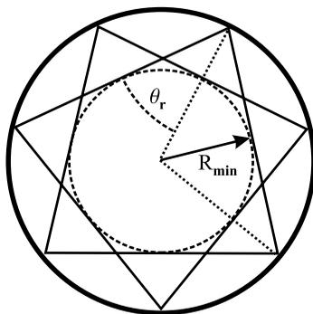
**Fig. 5.54** Transverse mode propagation through the disk center
