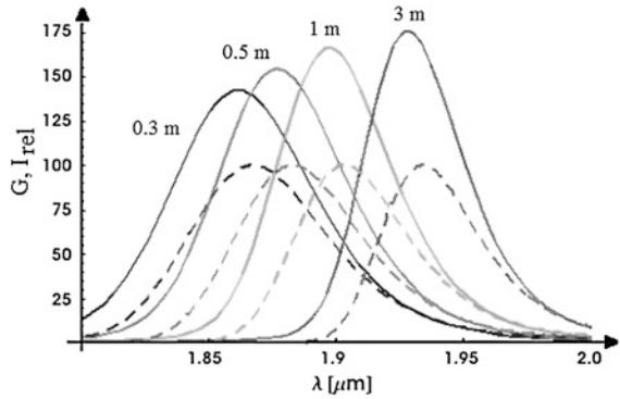
**Fig. 5.39** Measured fluorescence of a  $\text{Tm}^{3+}:\text{ZBLAN}$  fiber under excitation at 792–805 nm for different fiber lengths  $L$
