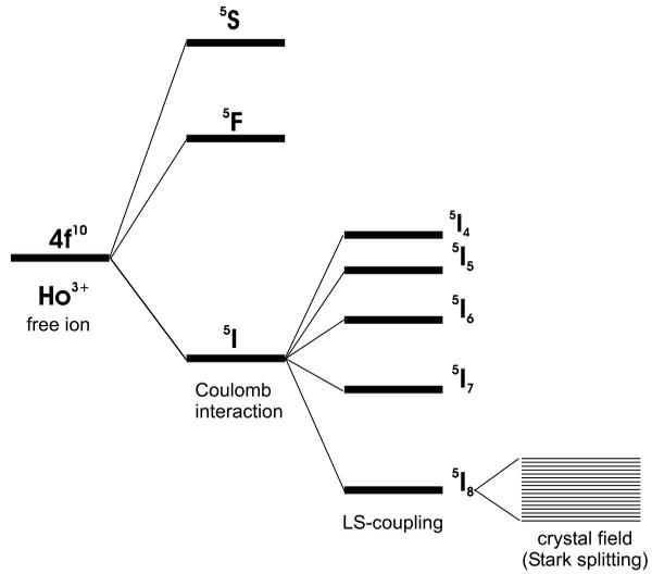
**Fig. 2.4** Quasi-three level scheme in a solid-state laser
